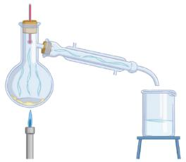
Salt water is heated up until it starts to boil, it is then cooled, condensed and collected. The salt is left behind in the flask and the pure water is collected in the flask.
