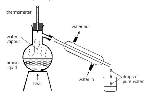
Water vapour from the brown liquid changed into drops of pure water which were collected in the beaker. What process caused the drops of water to form from the vapour? Tick the correct box.
